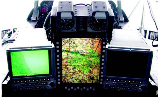
Figure 2. Tornado Navigator seat with TARDIS display (center) Image courtesy of BAE Systems
